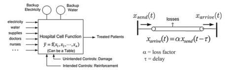
Fig. 12.6 Conceptual cell and channel models
