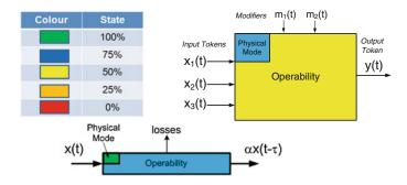
Fig. 12.7 i2Sim discretized cell and channel models
