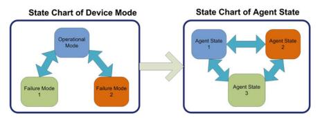
Fig. 13.15 Failure-oriented modeling approach
