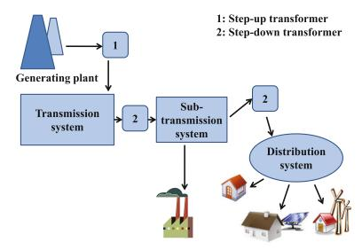
**Fig. 8.1** A block schematic of an electrical network. The *transmission system* operates at the highest voltage. The *sub-transmission* operates on medium voltage levels, while the *distribution system* operates on low voltage
