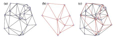
**Fig. 7.5** Each instance of the system is generated according to the following process: **a** First,  $N^{(1)}$  nodes (here  $N^{(1)} = 30$ ) are positioned at random within the unit disk and the Delaunay triangulation is produced; **b** the second network is then generated by drawing  $N^{(2)}$  (here  $N^{(2)} = 10$ ) nodes uniformly from the existing ones  $(N^{(2)} \le N^{(1)})$  and, once again, computing the Delaunay triangulation; **c** the combined system is no longer planar
