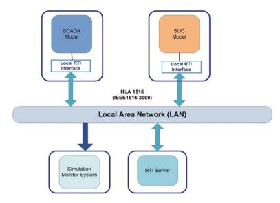
Fig. 13.14 Architecture of the experimental simulation platform
