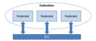
Fig. 11.9 Federation of simulators and Run-Time Infrastructure (RTI) middleware
