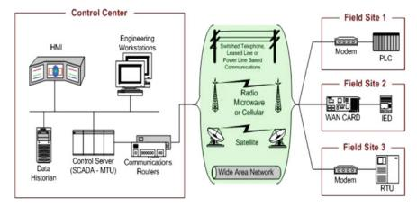
Fig. 13.2 General structure of a SCADA system [8]
