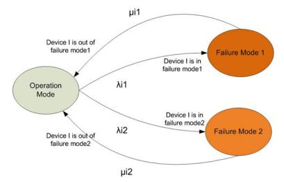
Fig. 13.16 State diagram of the device mode model ( $\lambda$  constant failure rate;  $\mu$  repair rate)
