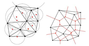
**Fig. 7.2** A Delaunay triangulation is a triangulation of points (*black dots*) in the plane where the circumcircle of each triangle does not contain any other points. If the centres of circumcircles (*red dots*) belonging to neighbouring triangles are joined together, the Voronoi diagram is produced (*red lines*)
