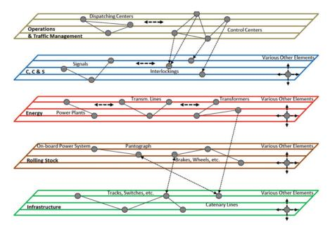
**Fig. 13.5** Multilayer representation of the railway system [18]
