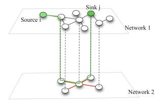
Fig. 7.3 Flows on two interdependent networks: edges of network 1 are shown in black, edges of network 2 are shown in red, and nodes in common to both networks are considered to be coupled (shown by *dashed lines*). Shown in *green*, we represent a path between two nodes, the 'source' i and the 'sink' j
