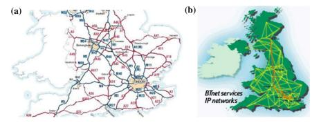
Fig. 7.4 a The national road network in England, and  $\bf b$  the network of major internet servers across the UK operated by British Telecom. These networks are consistent with planar subdivisions on a finite sampling of nodes taken with uniform density
