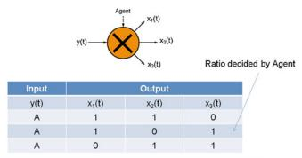
Assume for the example that we have an electrical substation with 3 feeders out and only 2 of them can be supplied.
