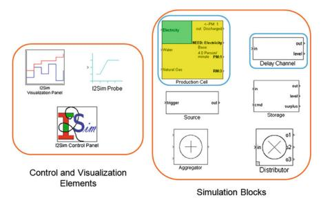
Fig. 12.15 i2Sim Toolbox for MATLAB/Simulink
