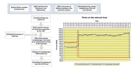
**Fig. 13.1** Initial conditions and failure mechanisms leading to splitting of the ENTSO-E grid on 4 November 2006 (formation of areas at 22:20; re-synchronization of area 1 and 2 at 23:24, of area 3 at 23:57 h) [3]
