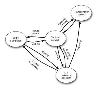
**Fig. 7.1** Types of interdependencies between different critical infrastructures—adapted from Ref. [1]. Failure in the water distribution network might cause disruption at a power station, due to lack of cooling. This, in turn, could affect control networks employed to monitor water distribution in the first place, exacerbating the initial failure
