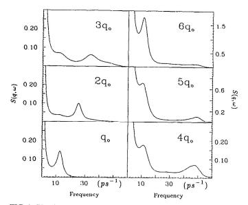
FIG. 1.  $S(q,\omega)$ , measured in arbitrary units for different q values (shown in units of  $q_0 = 0.3316 \text{ Å}^{-1}$ ), and shown as a function of  $\omega$  (in ps<sup>-1</sup>). The maximum entropy method (Ref. 9) was used to obtain these curves.
