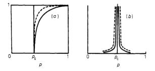
Figure 2. Schematic behaviour of backbone quantities (full curves) as a function of pure percolation quantities (broken curves). (a) shows the order parameters P and  $\overline{P}$ , while in (b) we sketch the mean size functions S and  $\overline{S}$ .
