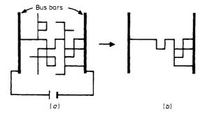
Figure 1. Bus bars are attached to the extremities of a cluster and a potential difference applied (a). Current flows in the backbone bonds (b), but not through 'dangling ends' which are attached to the backbone at only one vertex.
